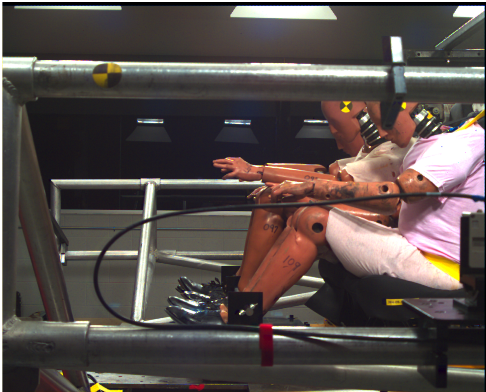
Figure 4 – Captured image from the sensor at 1000 fps, 80 msec after impact.
